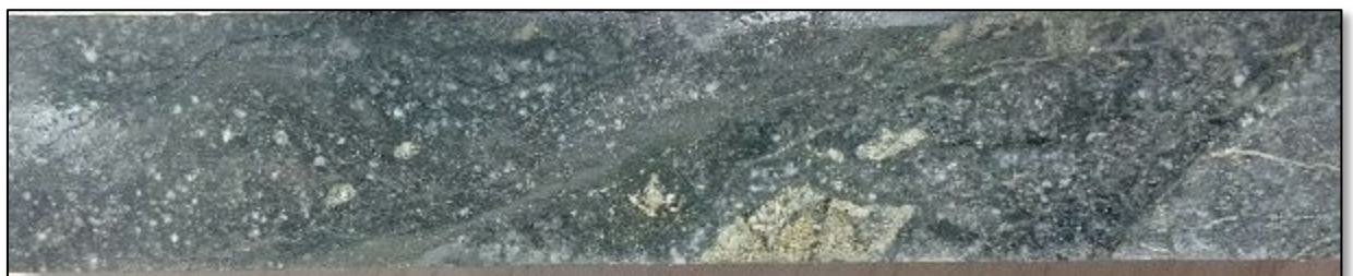
Figure 1. Pyrite-chalcopyrite-marcasite and magnetite veining with biotite alteration in sheared granodiorite.
