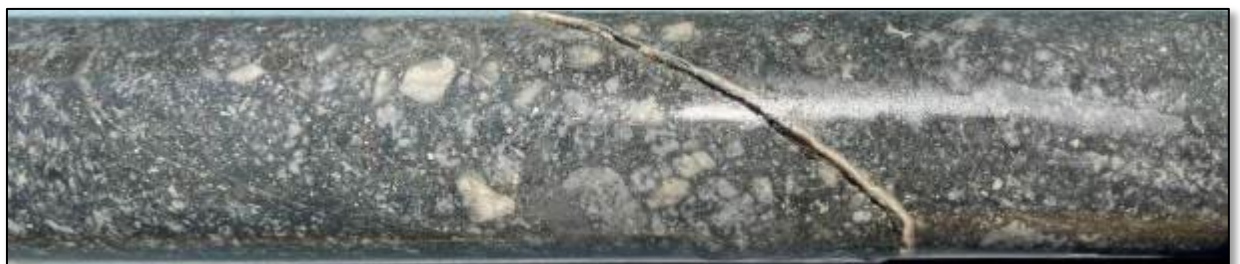
Figure 2. Polymictic breccia at contact between granodiorite and rhyolite. Biotite and pyrite matrix.
