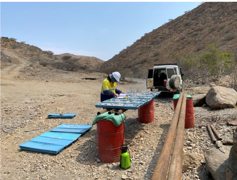
Figure 3: View towards the south of the logging site. Geologist Neil Scholtz logging drill-core from NDDH004.
