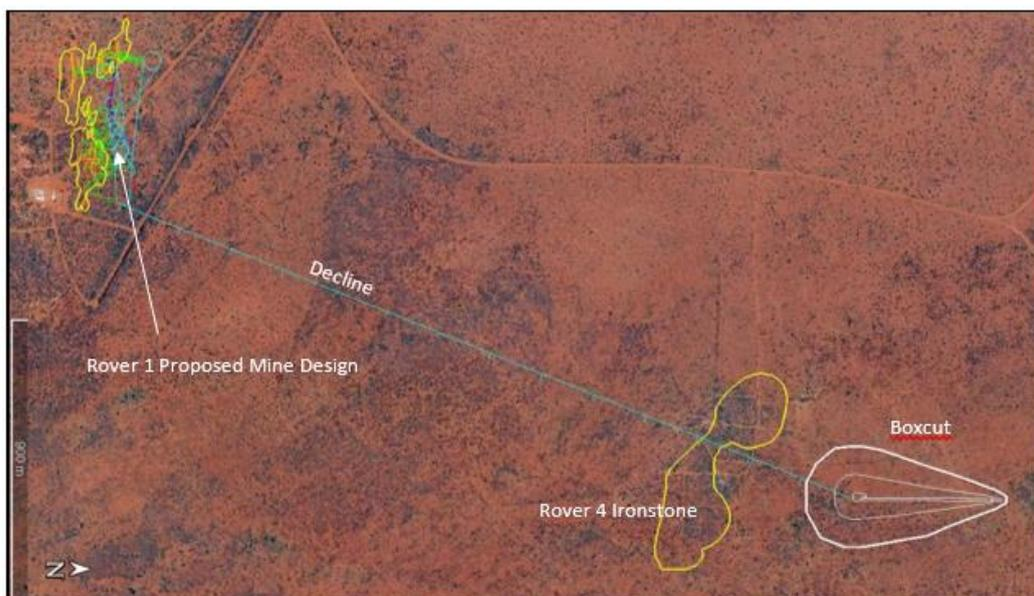
**Figure 1: Rover 4 Location below the planned Rover 1 Decline.**
