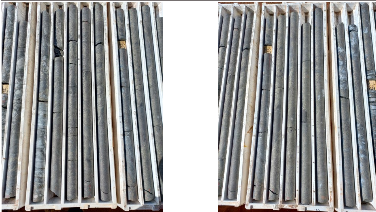
Figure 3 Hole NKLCSD001 from hole depths 444.2m to (LHS core block) to hole depth 456.8m (RHS core block) depicting typical semi-massive to massive pyrrhotite-marcasite/pyrite sulphide-quartz breccia textures encountered between 314m and 487m downhole depth.
