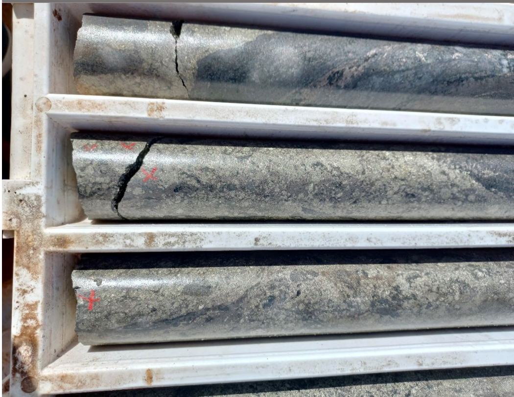
Figure 4 Hole NKLCSD001 detailed typical semi-massive to massive pyrrhotite-marcasite/pyrite sulphide-quartz breccia textures encountered (450m top to 452m bottom).
