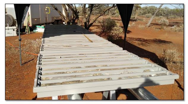
Figure 2: HQ core from the first day's drilling.
