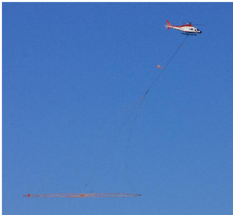
Figure 2: Helicopter towing the VTEM transmitter coil (courtesy UTS Geophysics).
