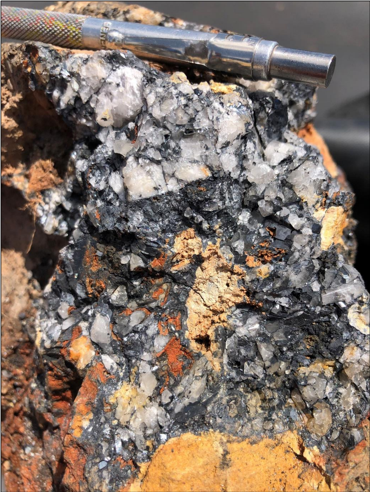
Figure 3: Photograph of quartz and manganese cemented siltstone breccia.
