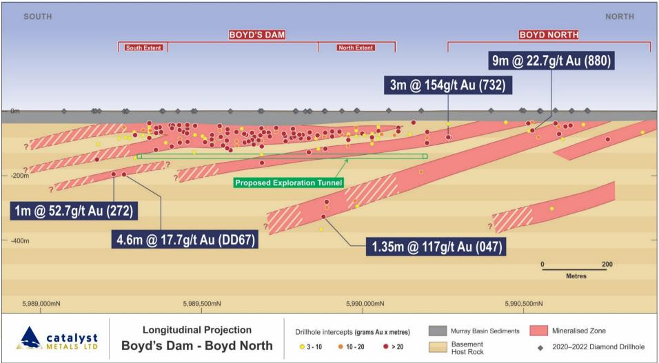
Figure 4: Boyd's Dam longitudinal projection showing proposed exploration tunnel
