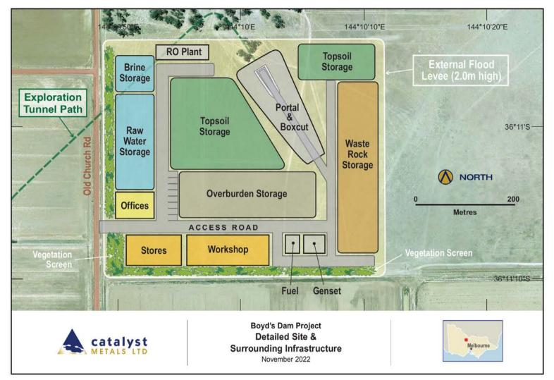
Figure 3: Boyd's Dam Detailed Site Plan
