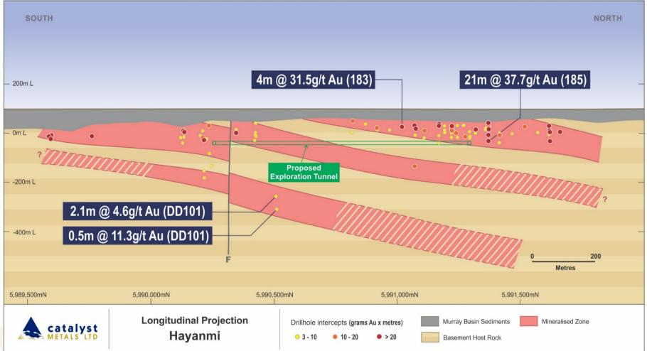
Figure 5: Hayanmi longitudinal projection showing proposed exploration tunnel
