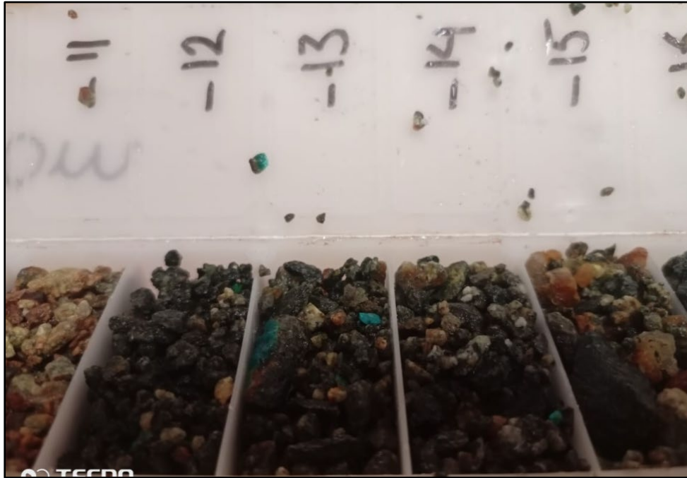
Image 2 / RC drill chips: 22CURC004 11m to 15m, 4m at 5,020 ppm Cu and 8,720 ppm Zn
