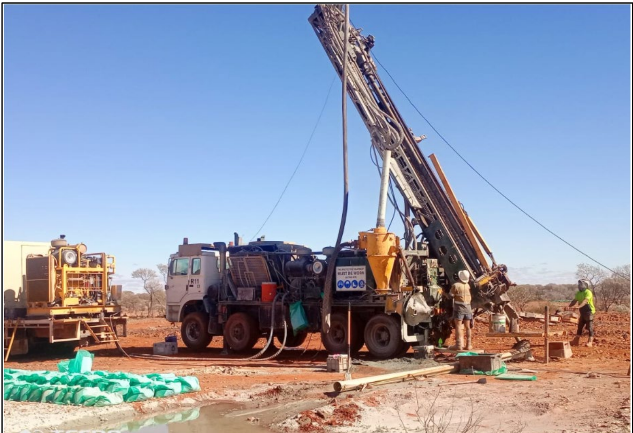
Image 1 / RC drill rig at Mt Eelya Cue/Murchison Copper Project, May 2022
