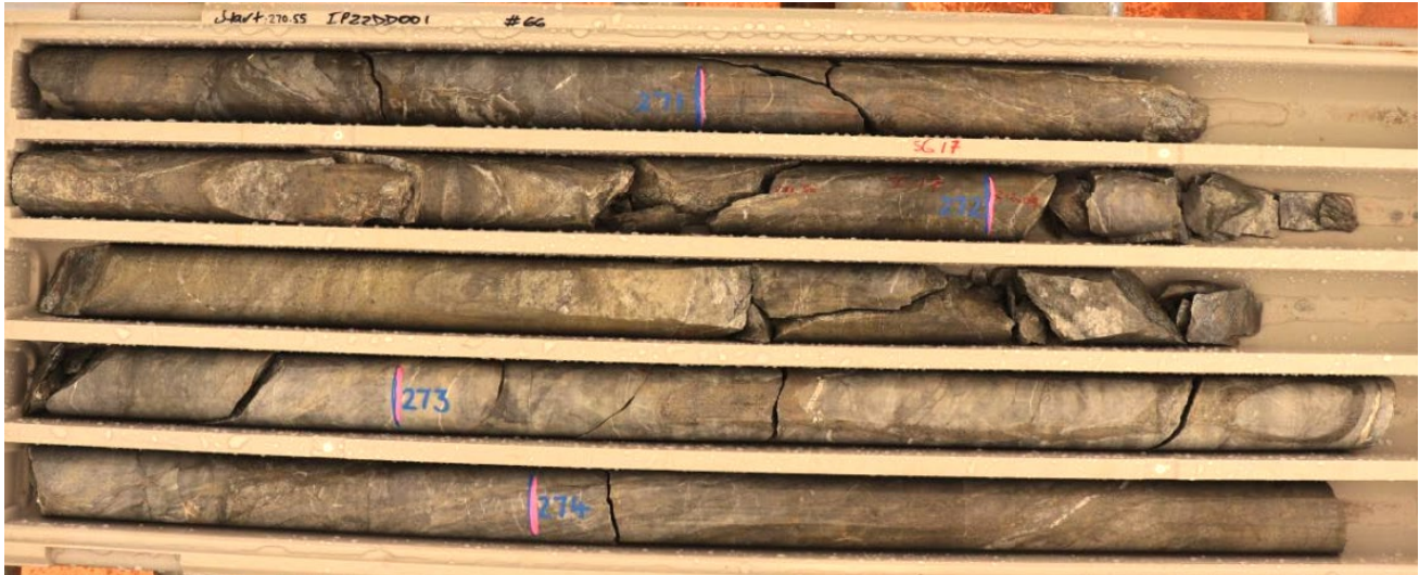
Figure 4 – Drill core IP001 – 271m down-hole photograph illustrating fine pyrite mineralisation and carbonate-sericite-silica alteration with veinlet, matrix and disseminated sulphide minerals, typical of the 13m section, in the interpreted position of the Rangoon Fault.
