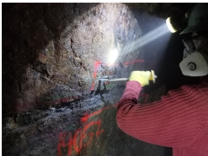
Figure 1 and 2. Underground and surface channel sampling. Note veining and brecciation in photo 2.
