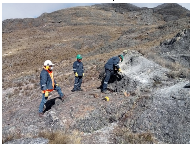
Figure 3. Surface sampling of a mineralised structure, cutting a continuous channel with a diamond blade.
