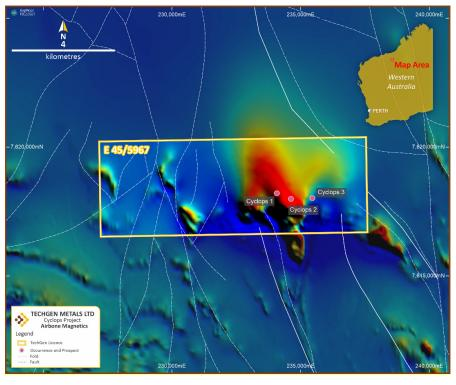
Figure 2: Airborne EM targets over magnetics, Cyclops Project.
