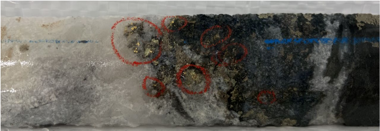
Figure 3: Photograph of the quartz vein margin of the intersection grading 0.4m @ 1,020g/t gold. Drill core size is NQ.
