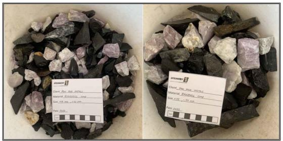
Photo 1. RKDD006: Sub-sample of crushed core feed for ore sorting, LHS +10mm to -25mm RHS +25mm to -50mm
