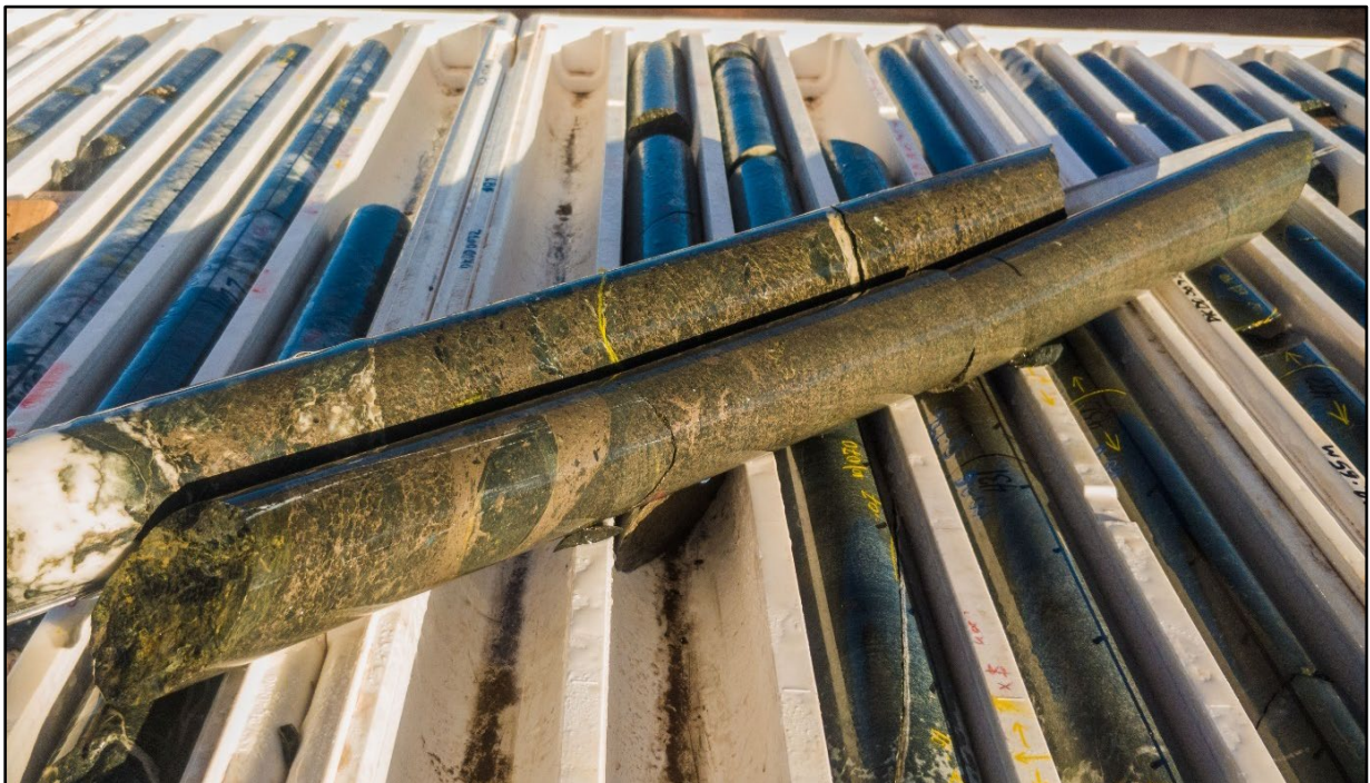
Figure 1: DKDD0032 sulphide intersection 428.1-429.4m – heavily disseminated/matrix sulphides in ultramafic.
