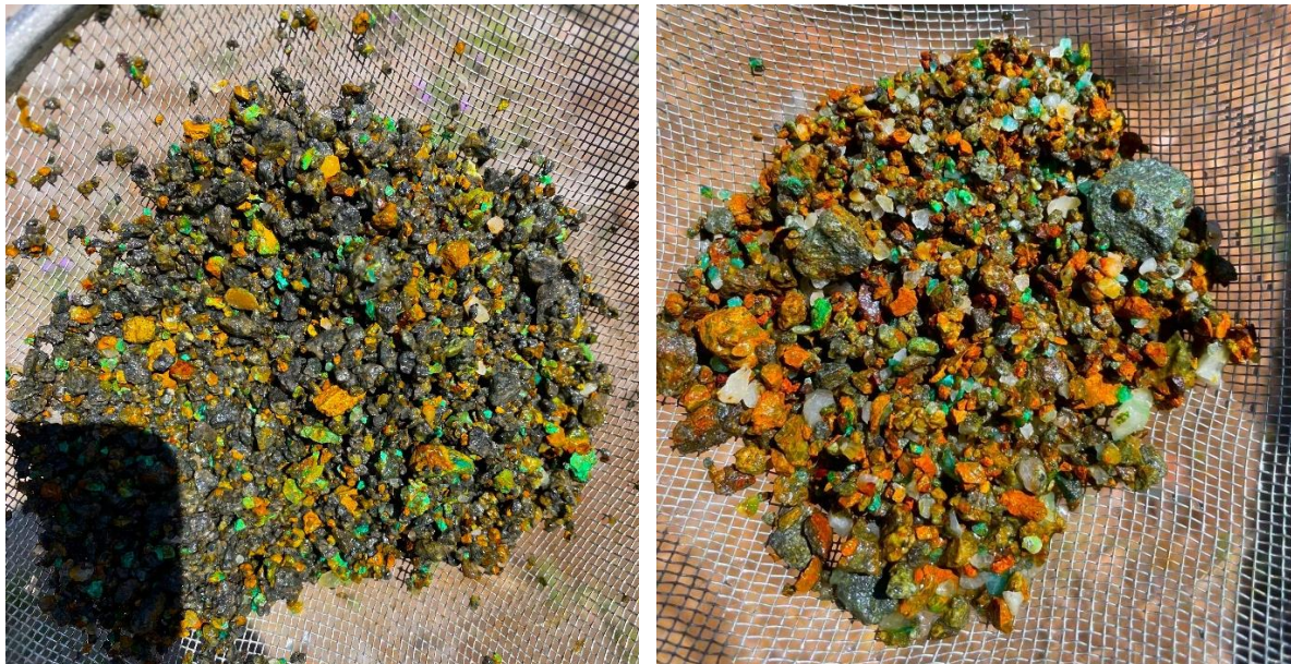
Figure 1. (Left) BIM011 21-22m with 10 % of malachite and 10% quartz (visual estimate) and (Right) BIM010 11-12m with 5 % of malachite and 30% quartz (visual estimate) – refer to Table 1
