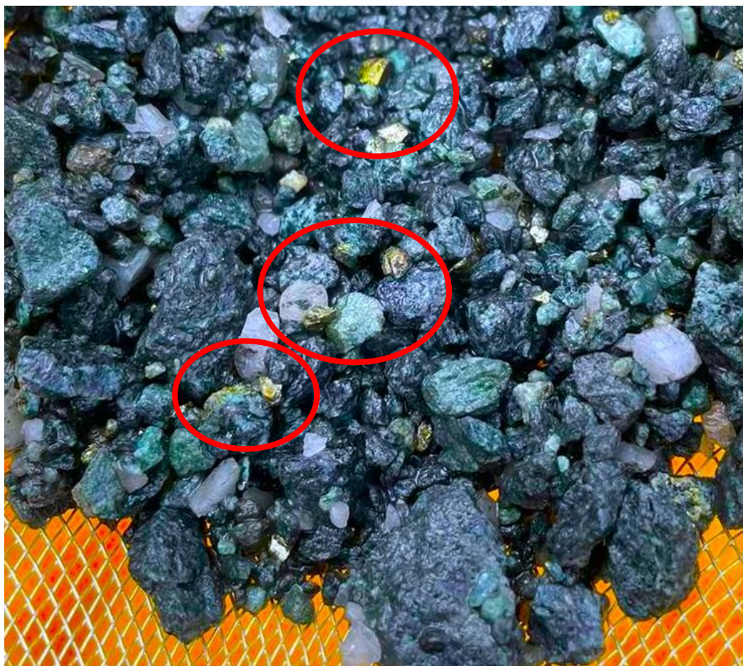
Figure 2. Chalcopyrite in BIM005 from 29-30m with visual estimate of 1-3% chalcopyrite (highlighted in red circle) and 40% quartz
