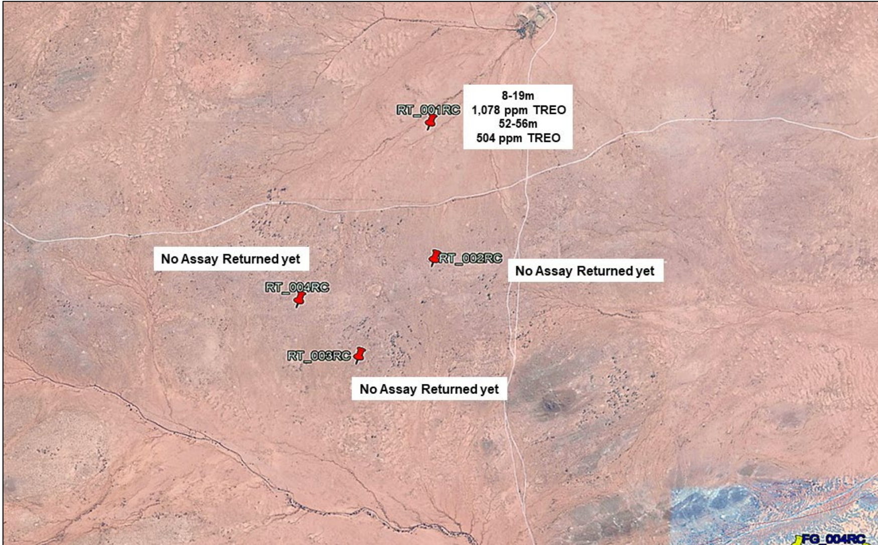
FIGURE D1-3: REEFS TANK DRILLHOLE LOCATION AND TREO RESULTS NOVEMBER 2022
