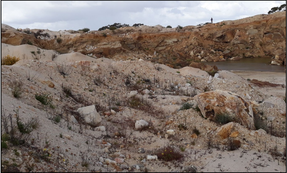
Figure 4. Historic Quarry at the Karloning Project showing pegmatite and the host granitoid in the quarry wall.
