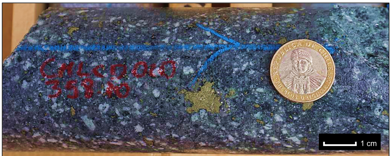
Figure 4: 169 metres at 1.08% Cu and 225ppm Mo returned from drillhole CMLCD010 (Photo 358-359m).
