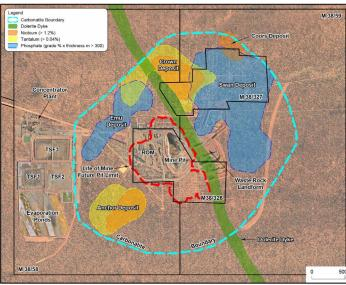
Figure 3 Mt. Weld Carbonatite (MWC) and related mineral deposits. Rare Earth Elements (REE) mine pit and 20 design of the future pit limit (red outline) is confined to the saprolite zone of the carbonatite
