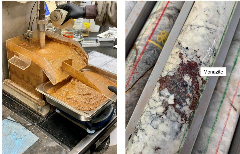
High quality concentrate from preliminary work: 12.3% Nd2O3 / 40% TREO with 92.8% recovery – Significant metallurgical study underway
