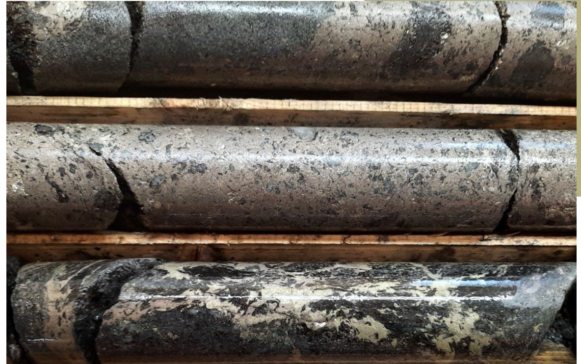
Discovery hole WAP22-003 interval comprises coarse grained pentlandite, chalcopyrite and pyrrhotite Source: Azmut Exploration
