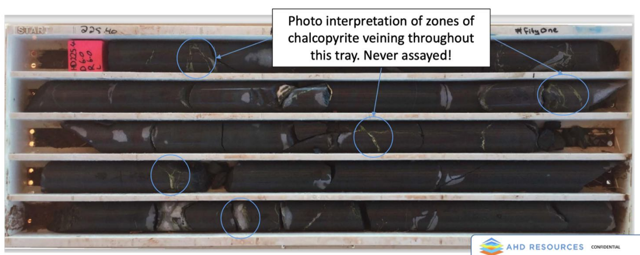
Figure 5: KCDD19001 GSWA core photo of Tray #51 with interpreted Cu sulphide mineralisation
