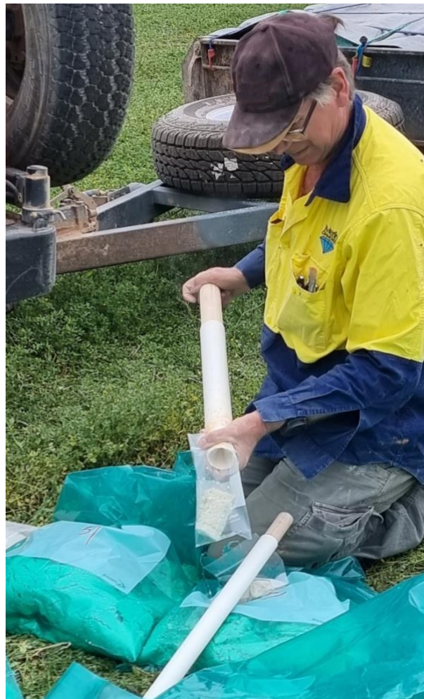
Figure 6. Onsite spearing of sample for lab analysis
