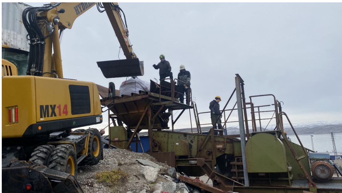
Figure 4: Crushing material from the Ivigtût waste dumps in Greenland down to 30mm.
