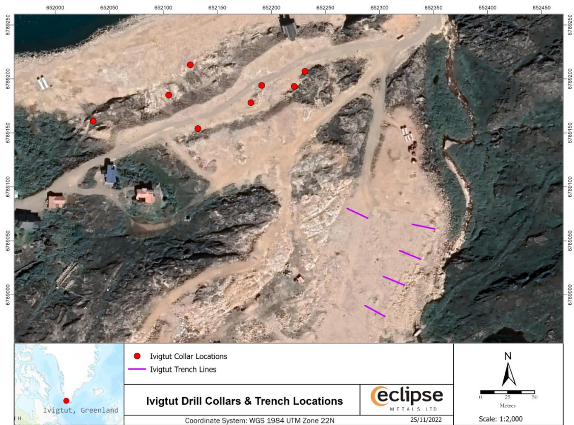
Figure 3: Ivigtût target area. Drill collars are marked with red dots. Bulk sample trenches are marked with purple lines. Assays are expected to be available toward the end of Q1 2023.
