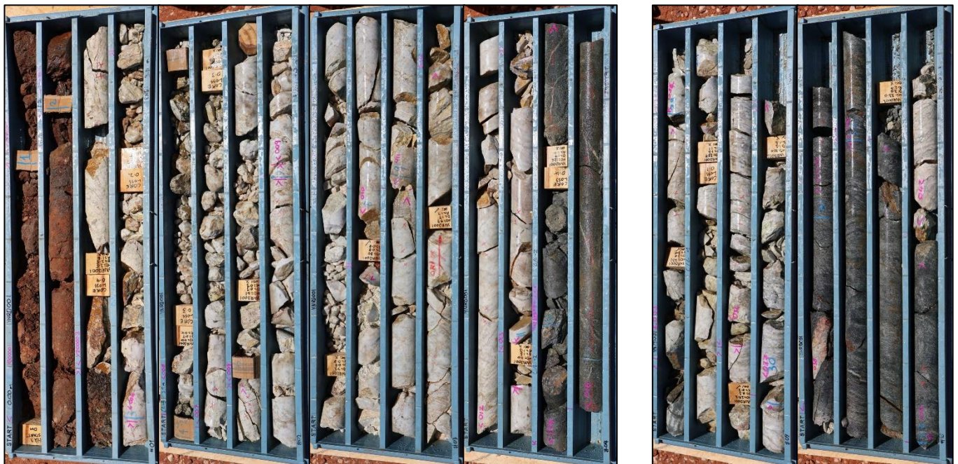
Figure 6: Photo of YNRD001 showing pegmatite intercepts from 2.5m to 11.7m and 27.6m to 30.4m.
