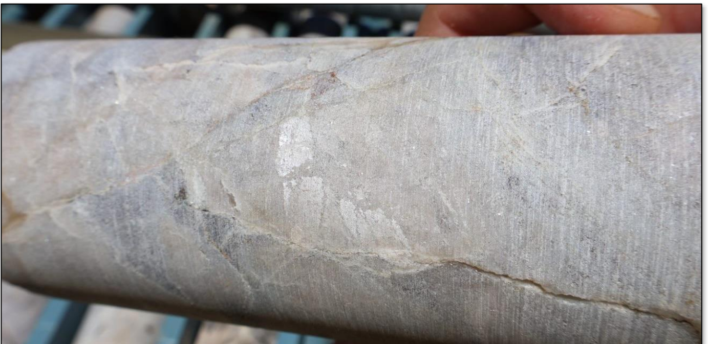
Figure 8: Close up photo showing coarse spodumene with 1-2mm spodumene disseminated throughout in YNRD002 from 28m.
