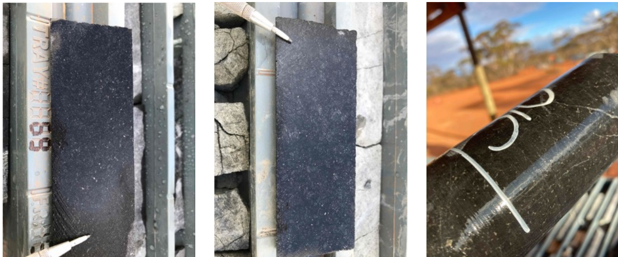
Figure 5: Photos of core from hole MTD020 showing disseminated sulphides that coalesce into interstitial blebs between olivine grains
