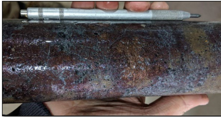
Photo 3. An uncut face of HQ3 diameter drill core from 85.3m drill depth in SMD050. Note the dominant copper sulphides being bornite (purple) and chalcocite (gun metal grey).
