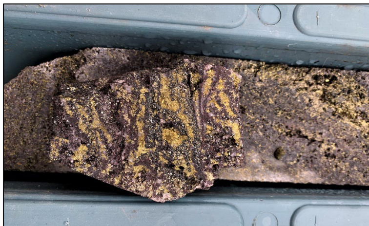
Photo 6. Chalcopyrite-specularite-hematite-magnetite mineralisation - SMD182, 423.5m drill depth, HQ3 diameter ½ cut drill core.
