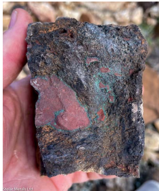
Figure 1: Left: View of the historical Line of Lode at Baratta Copper Mine, Right: Example of discarded copper ore on old working within the granted EL (XRF: 36% Cu and 478 g/t Ag)
