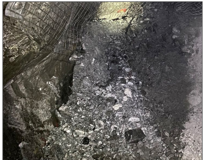
Figure 2: Fired stope (2005 Level), noting massive nickel sulphides (LHS wall)
