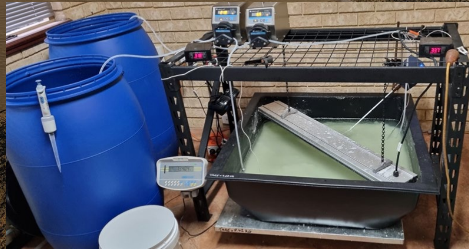
Leonite precipitation set-up
