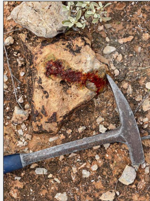
Zinc-zap wet chemical test highlights high-grade Zn
