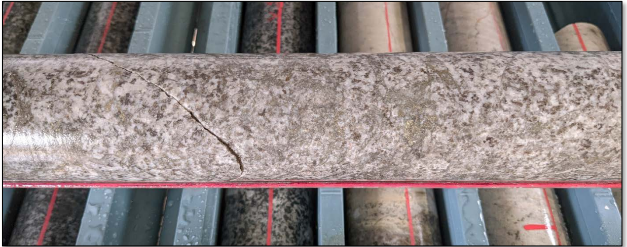
Figure 2. Intense biotite-albite-pyrite altered granodiorite near contact of rhyolite (cream coloured core in tray) and host granodiorite. Core photographed is from 495.4m.
