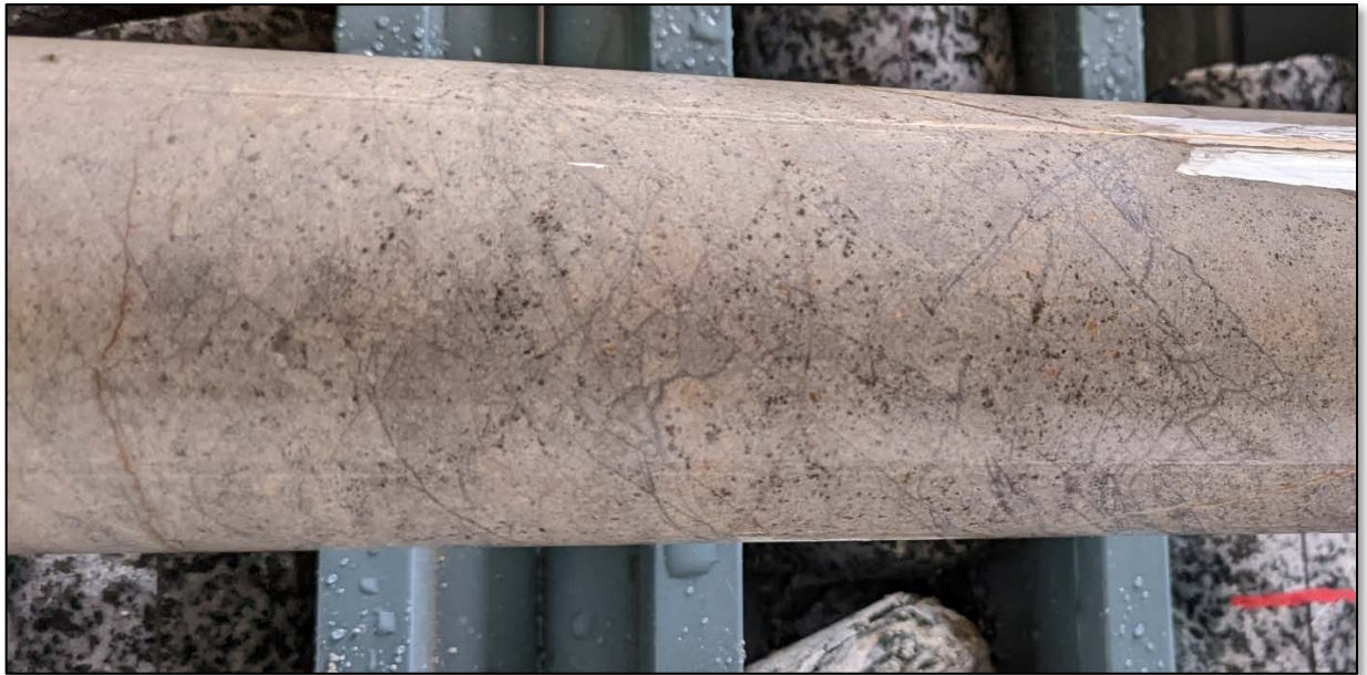
Figure 4. Crackle brecciated rhyolite containing pyrite predominantly in fractures. Core photographed is from 492.8m.
