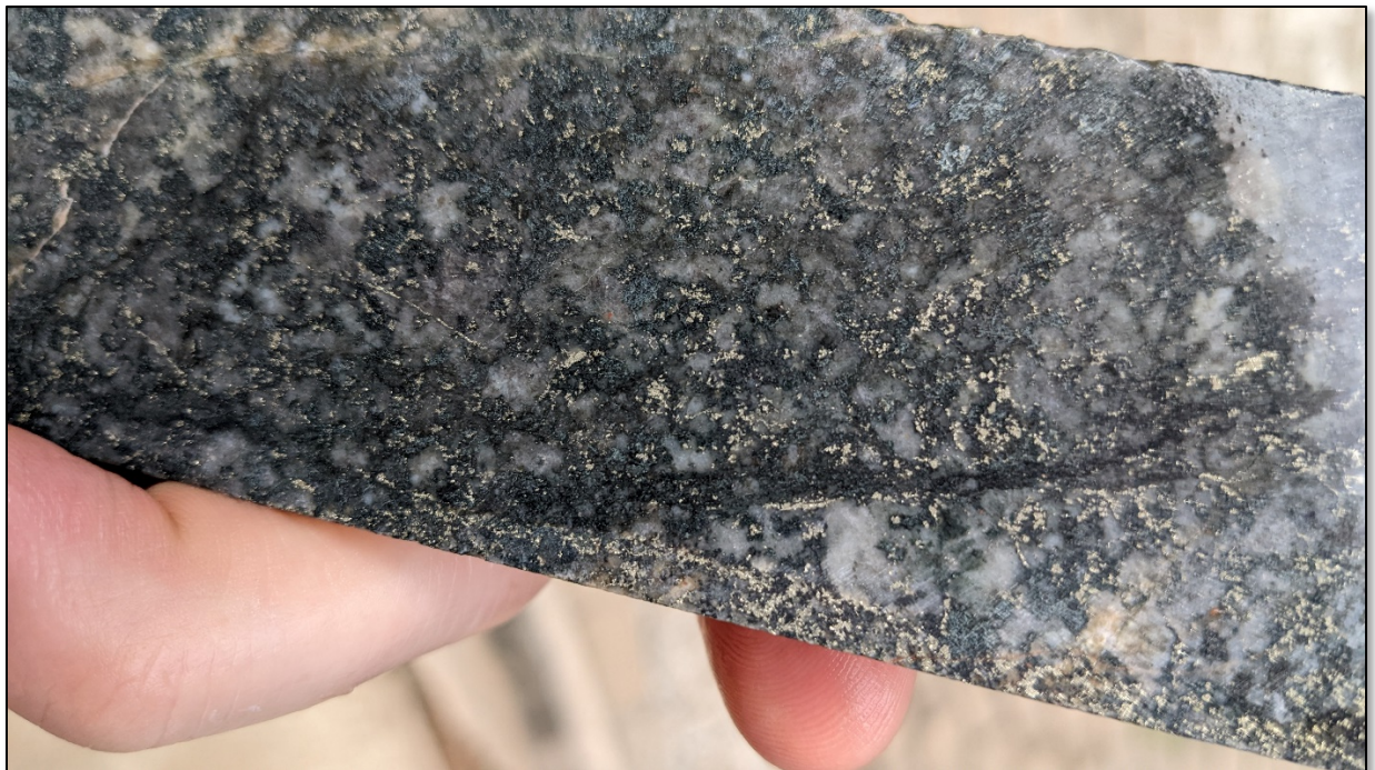
Figure 3. Magnetite vein in biotite-chlorite altered granodiorite with abundant pyrite. Core photographed is from 601.5m.
