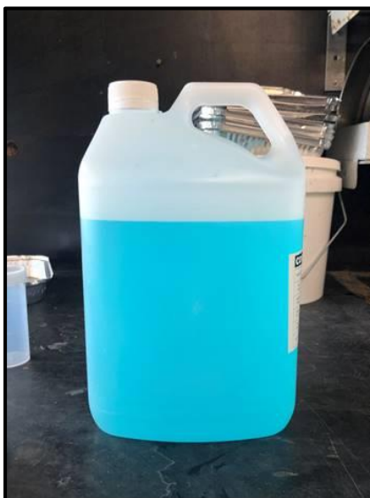
Figure 5: Green Hill Bottle Roll Leachate Solution with Blue Colour Due to Copper in Solution
