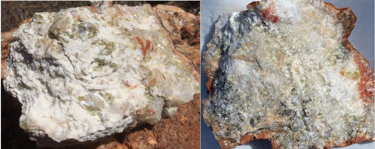
Figure 3 – Left Sample MW2211_15 and Right Sample MW2211_37. Both are micaceous Pegmatite samples from the western margin of Target 1. Both samples exhibited geochemical responses of LCT pegmatites.
