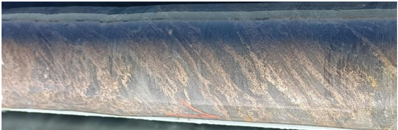
Image 2: Semi-massive sulphides (Po, Cpy, Pn) in SBDD005 at 343m downhole, HQ core.
