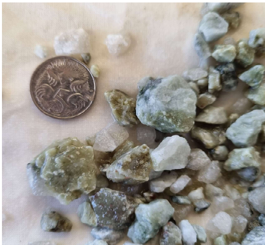
Figure 1: Lime green to grey spodumene with white albite and quartz, drill hole ECRC009
