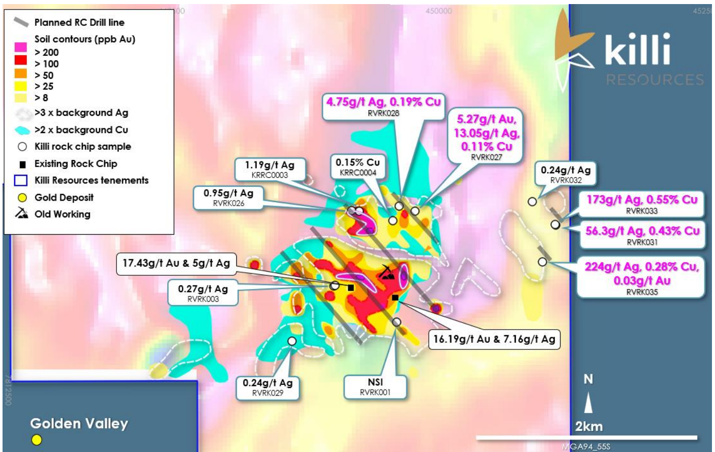
Figure 2. Location of rock chip & soil results at Rocky prospect. Soil results are contoured for various levels on gold mineralisation, copper, and silver, with the location of historical and recent rock chip samples, old workings, overlaying the magnetics from the recently flown VTEM survey.
