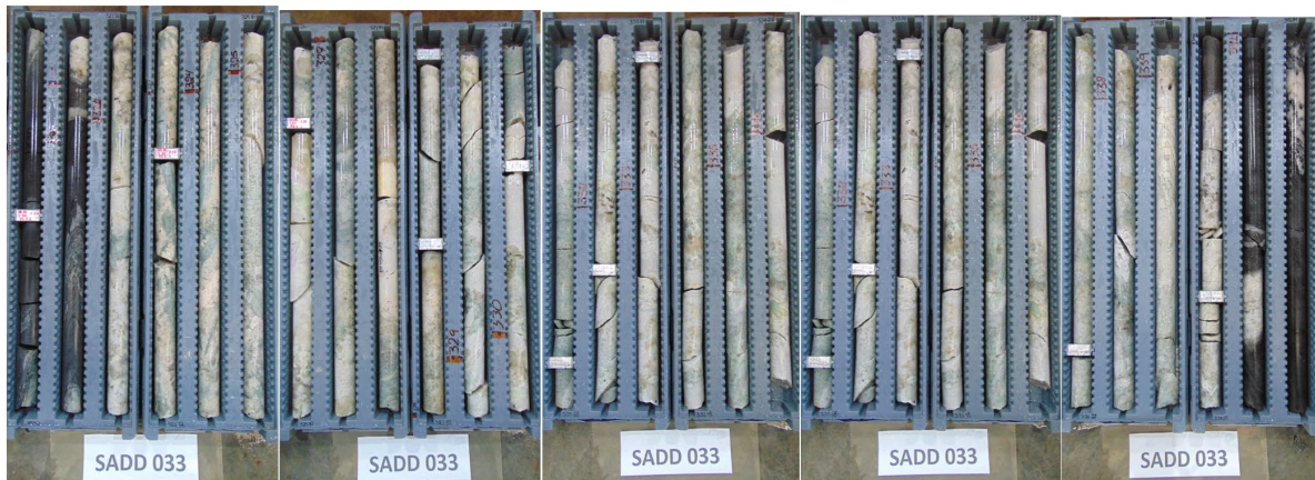
Figure 2: Colina West drill hole SADD033 – pegmatite intersection 319.40m – 341.94m (18.71m @ 1.32% Li 2 O 2 )
