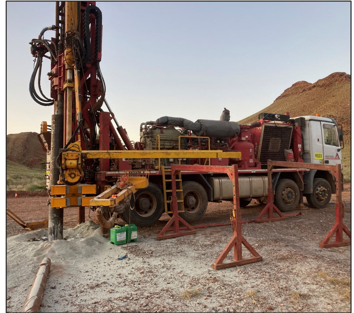
WATER BORE RIG ON SITE DRILLING BORES
