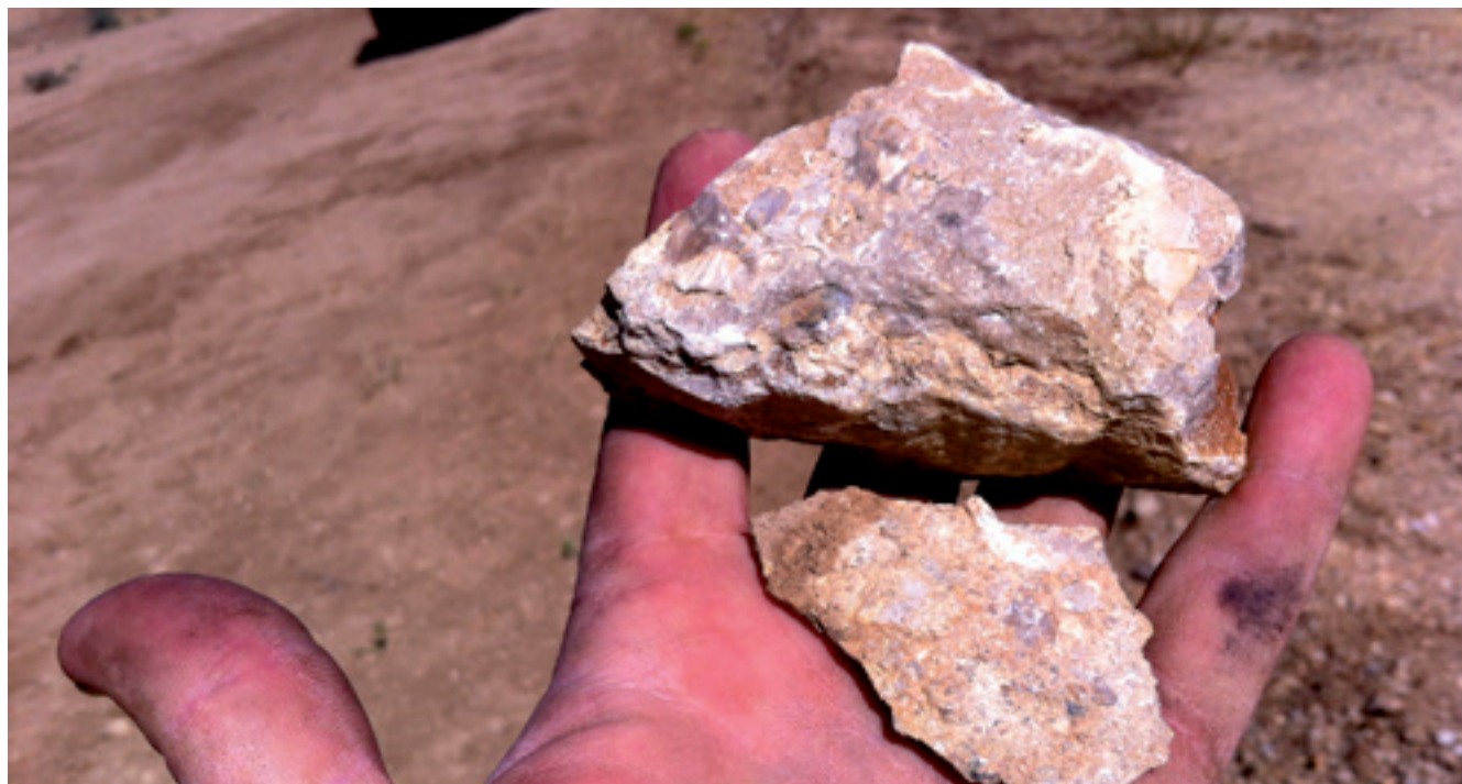
Figure 7 – Typical oxidised shale free of organics, crumbly nature, easy to process
