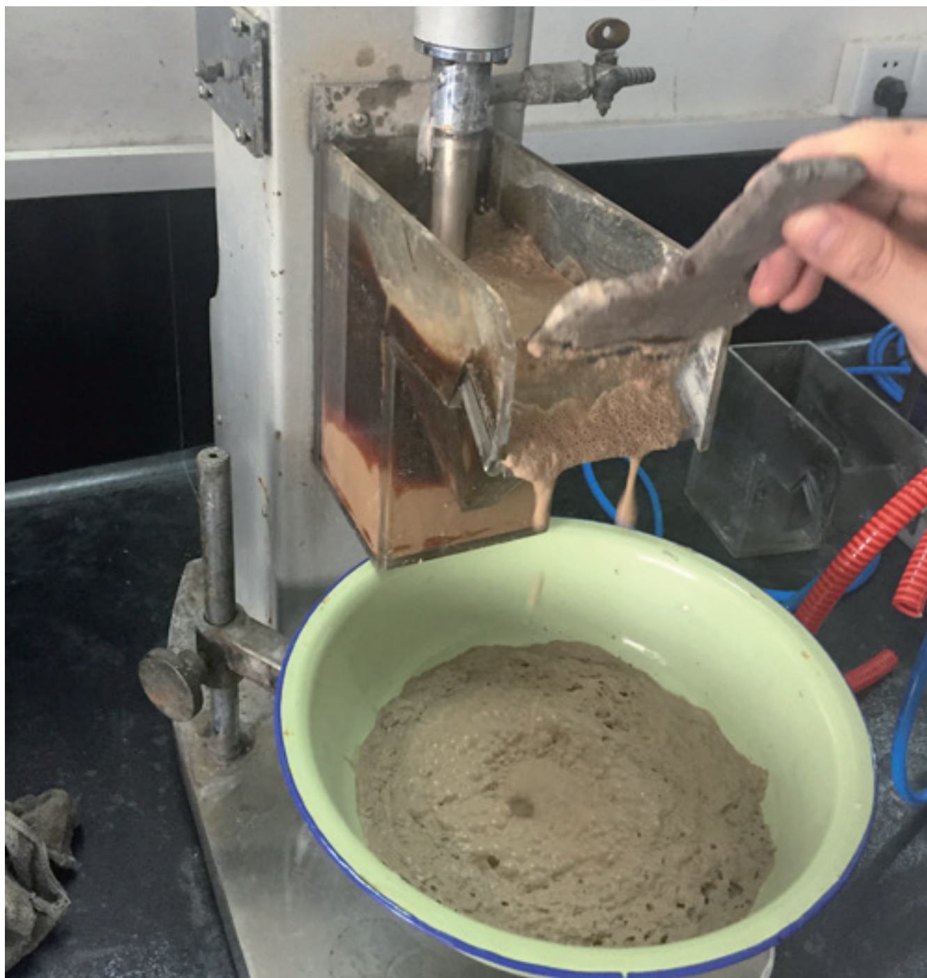
Figure 11 – Flotation Testwork undertaken as part of the vanadium concentration process
