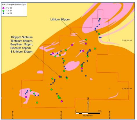
Figure 4 - Brisk Area 1 anomalous lithium samples with indicator elements
