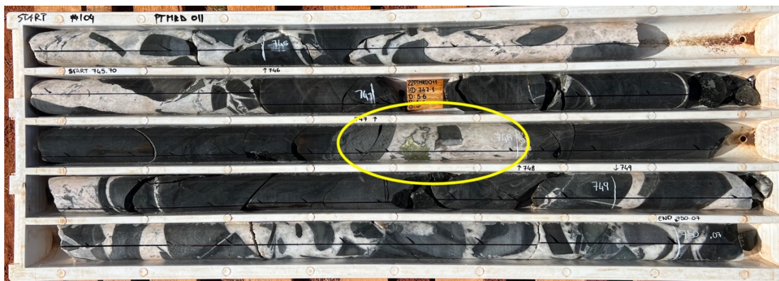
Figure 8: Hole 22PTMRD011 from 745.70 - 750.07m showing typical quartz – carbonate matrix supported jigsaw breccia that is dominate in the hole. Large slug of Chalcopyrite at 747.90m (yellow). Multi-element assays pending.
