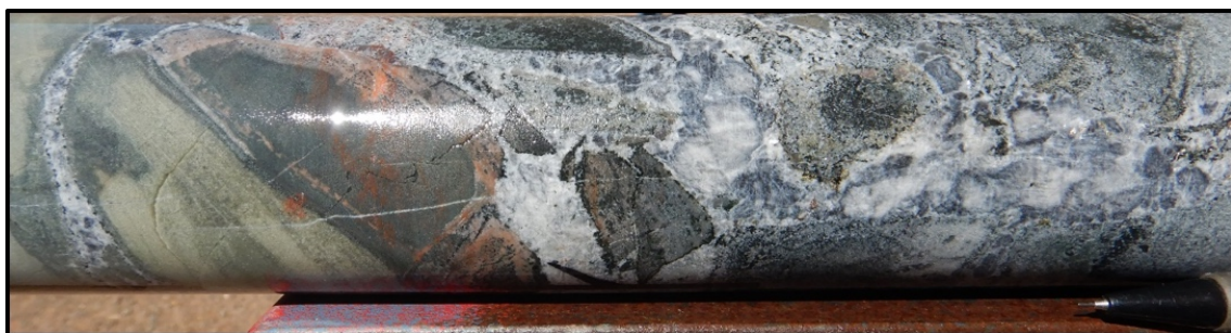
Figure 11: Hole 22PTMRD011 interval 773.7 – 773.9m showing a close up of the fluidised breccia. Note that some clasts have been reabsorbed into the matrix, while later incorporated clasts are sub-rounded. Minor sulphides are noted in the matrix. Wall rock exhibits sericite alteration with minor albite overprints.
