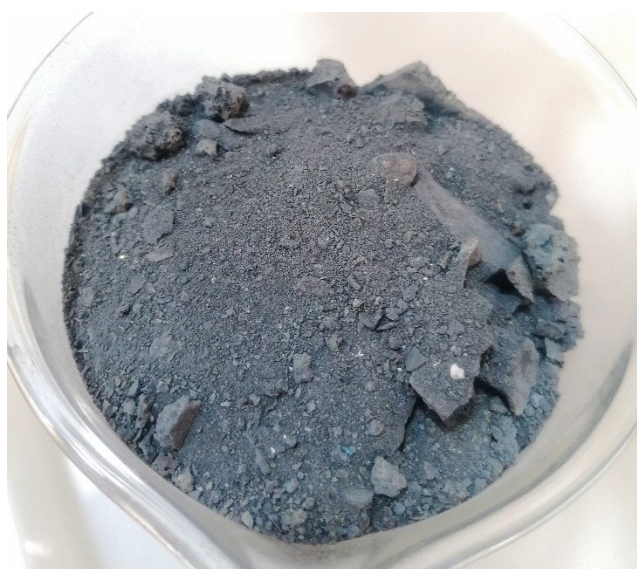
Figure 1: Feedstock (swarf) sourced from NdFeB metal alloy production, rich in Nd and Dy only.
