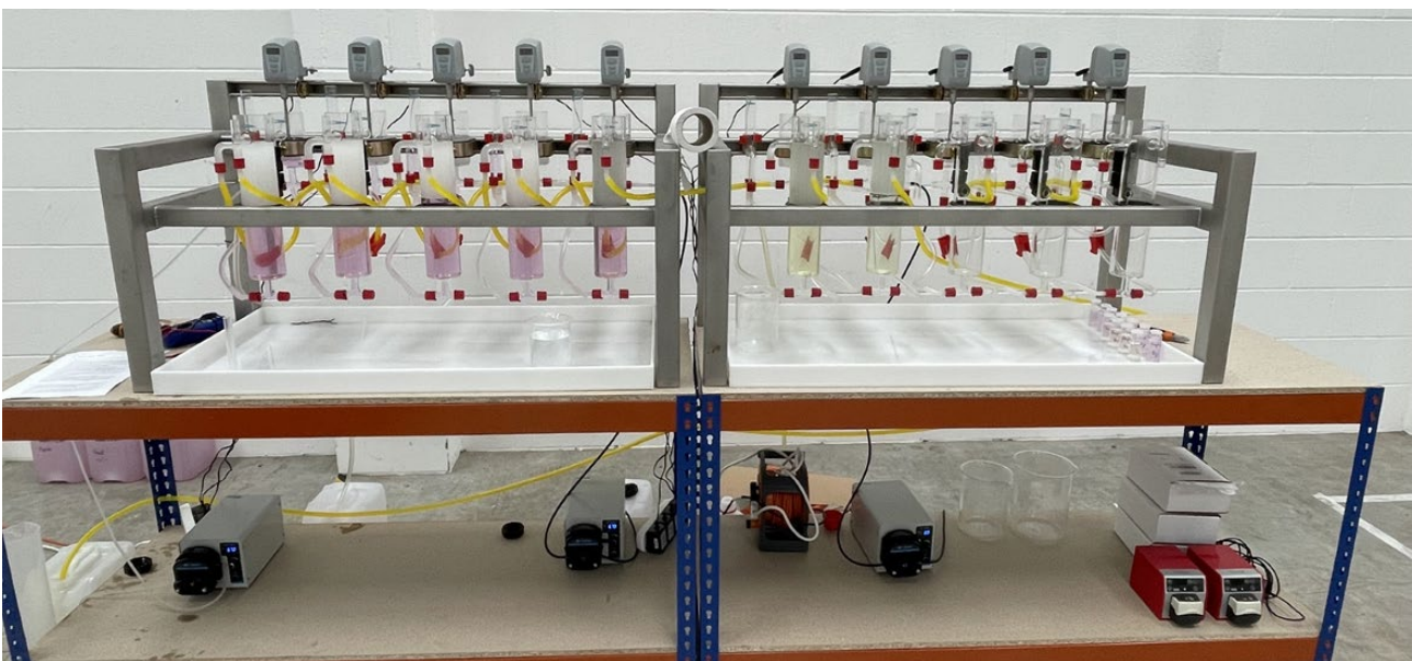
Figure 3: Mixer-settler circuit as part of the magnet recycling pilot plant. The first 5 stages show the separation of Neodymium (Nd) from Dysprosium (Dy) in the last two stages.
