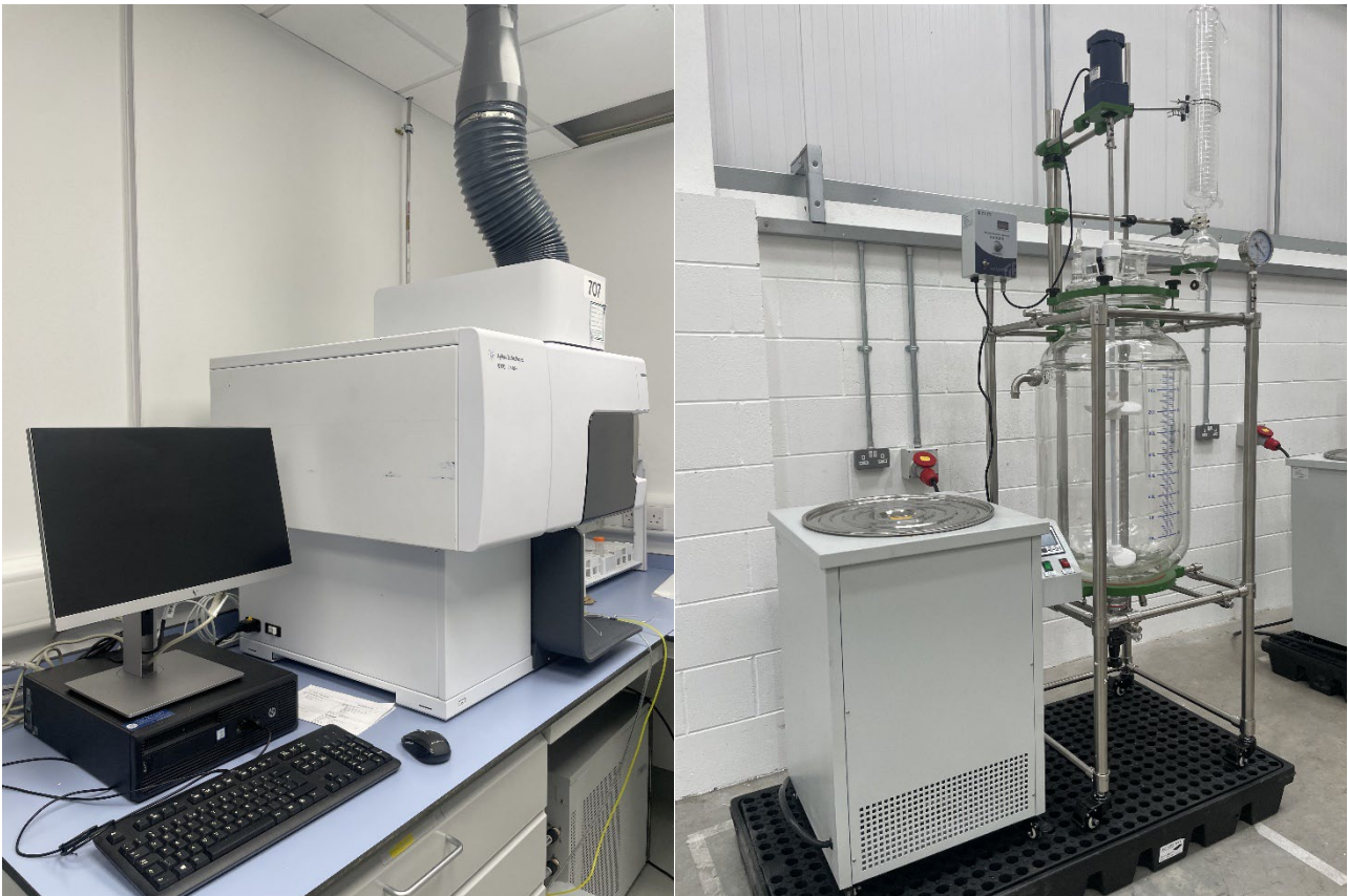
Figure 7: Left, analytical laboratory now operational with two (2) Inductively Coupled Plasma mass spectrometry (ICP-MS) instruments, and right, temperature-controlled glass process reactors being delivered for the demonstration plant.
