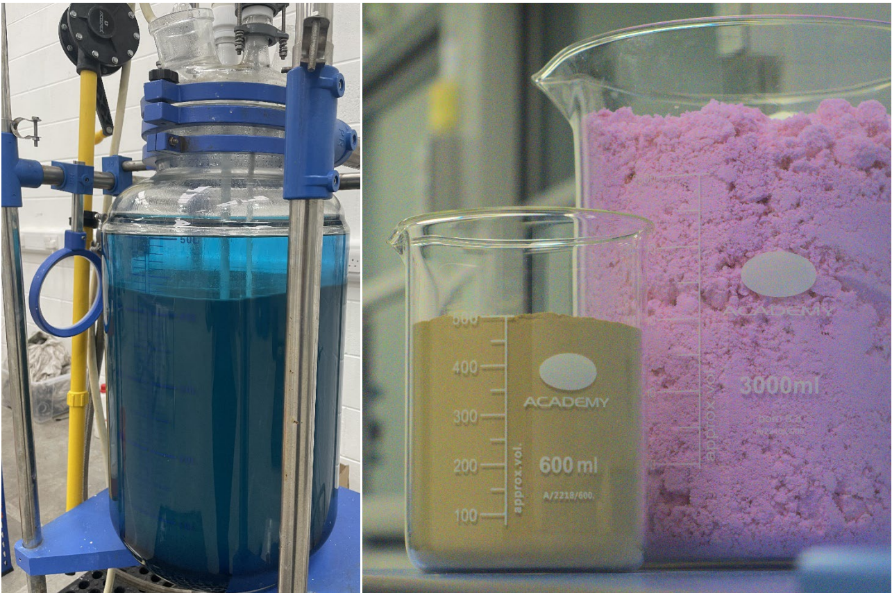
Figure 2: Swarf processing in reactor on left, prior to production of intermediate products – mixed Nd/Dy oxide (brown) and mixed Nd/Dy oxalate (pink), right.
