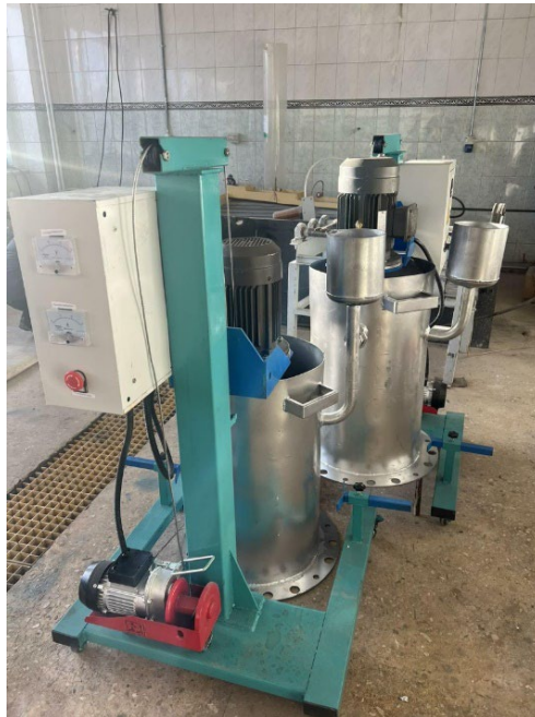
Image 3: Reagent mixing tanks Source: Temarise
