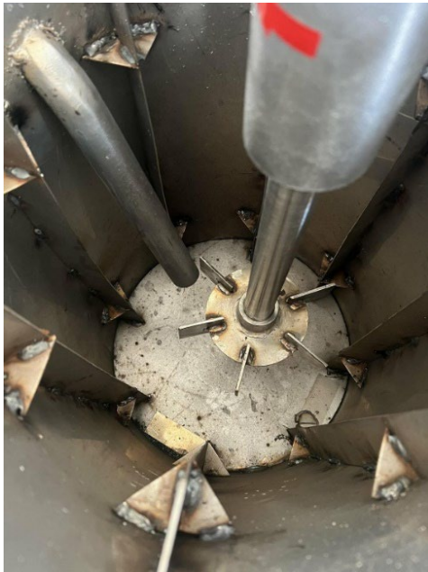
Image 4 & 5 Flotation tanks and high-speed mixers Source: Temarise
