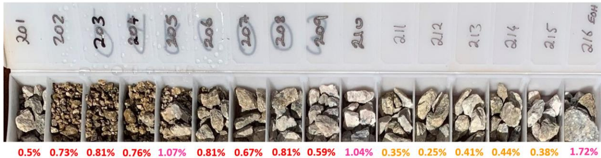
Figure 3: Chip Tray with Nb 2 O 5 Assay results annotated
