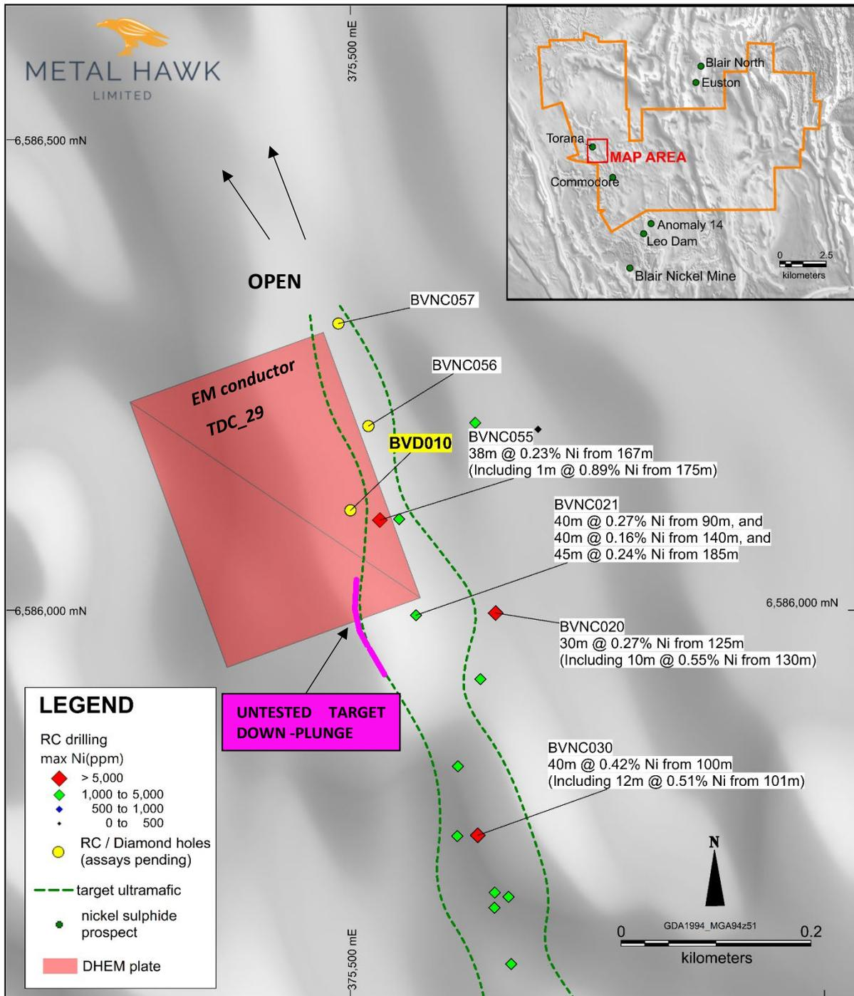
Figure 1. RC and diamond drilling at Torana
