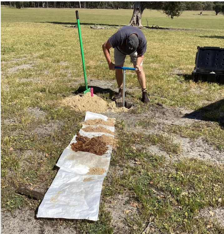
Diagram 3: Pictures of the hand auger drilling process, including restoration of the drill holes.
