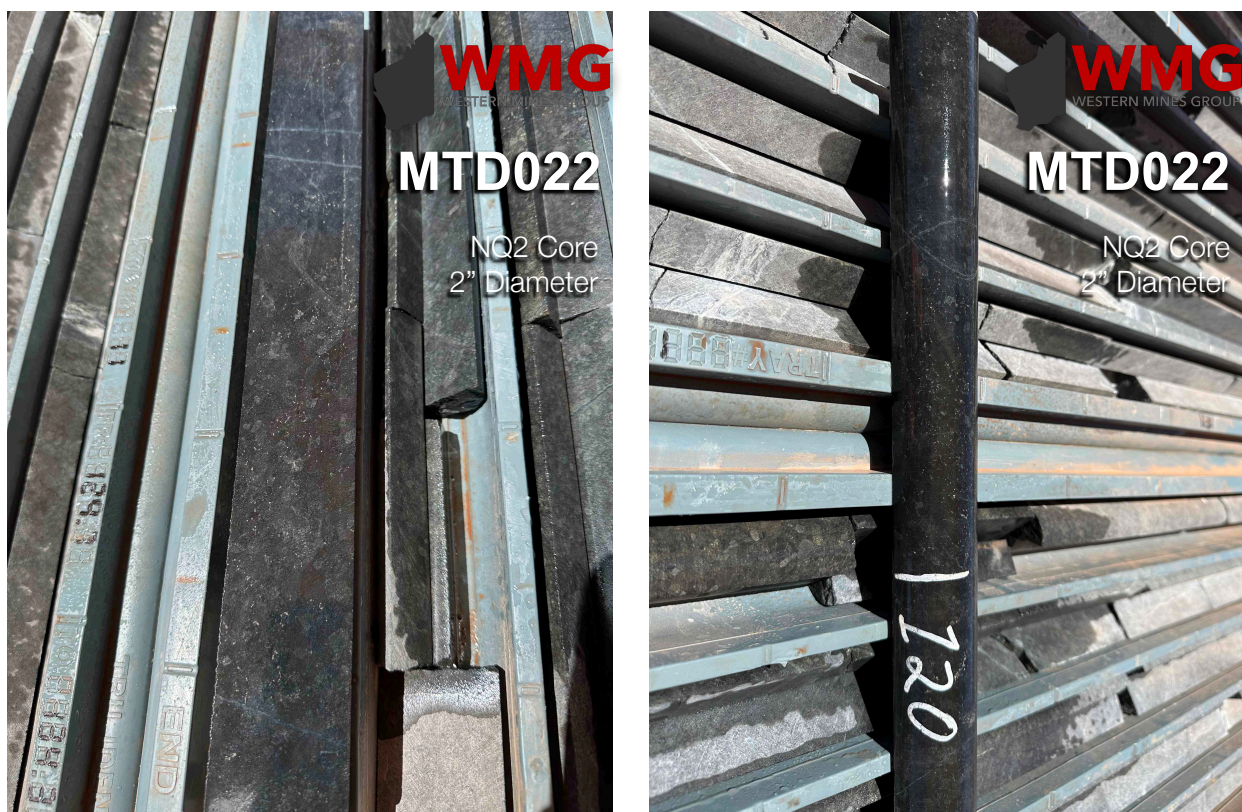
Figures 2A and 2B: Photo showing examples of visible disseminated sulphides in hole MTD022 with disseminated sulphide forming interstitial blebs between olivine grains
