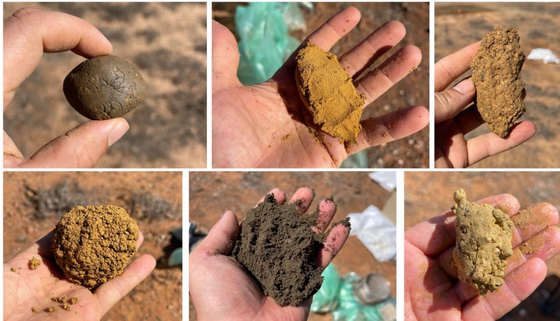
Figure 9. Examples of clays intercepted in the deep weathering profile in multiple RAB drillholes during the recent drilling at Morgans Creek.
