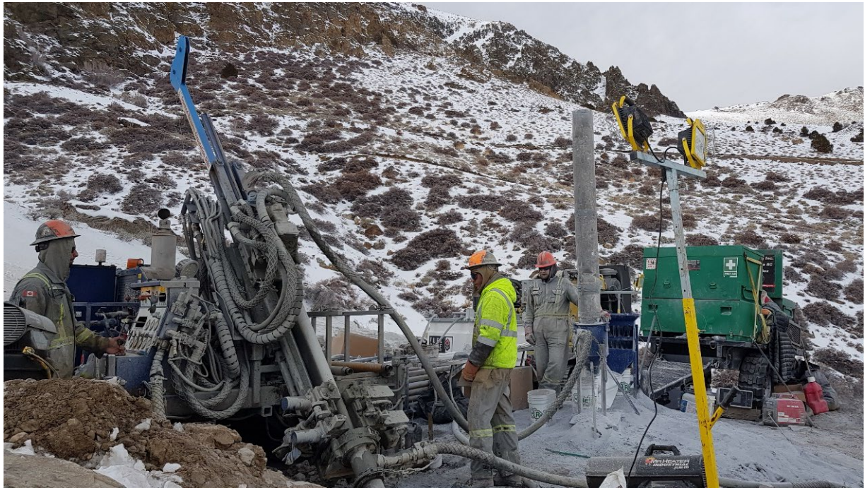
Figure 4. RC percussion drill rig on site drilling the first hole at Star Canyon, Nevada, December 2022.
